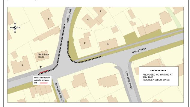
The proposal was designed to protect the sight lines on exiting North Lane and the vehicle access to North Back House.
